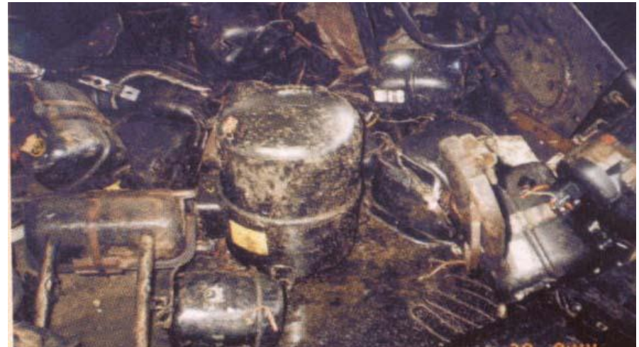
Contoh Limbah B3 impor yg mengandung Polychlorinated Biphenyl (PCBs). Dokumen Impor →skrap logam
